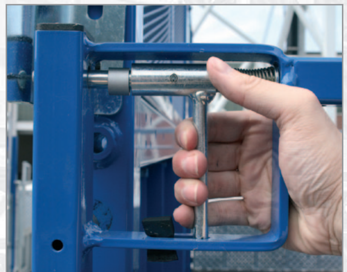
Safe locking of gates by a simple mechanism
